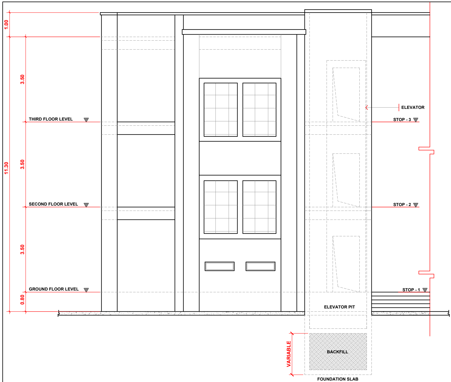
ELEVATOR FRONT ELEVATION SCALE: 1 : 80 MTS.
