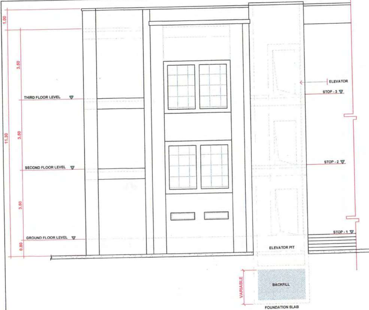
ELEVATOR FRONT ELEVATION SCALE: 1:80 MTS.
